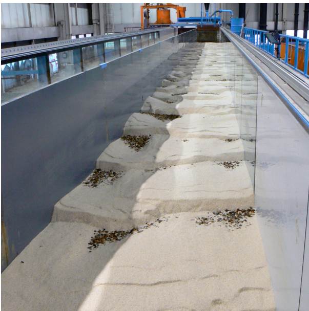
Photo 4.1: This photo shows a flume experiment with a supply-limited condition. The immobile gravel layer shows in the dune troughs. The limited sand presence causes reduced bedform dimensions, a decreased bed roughness and sediment transport rate.
