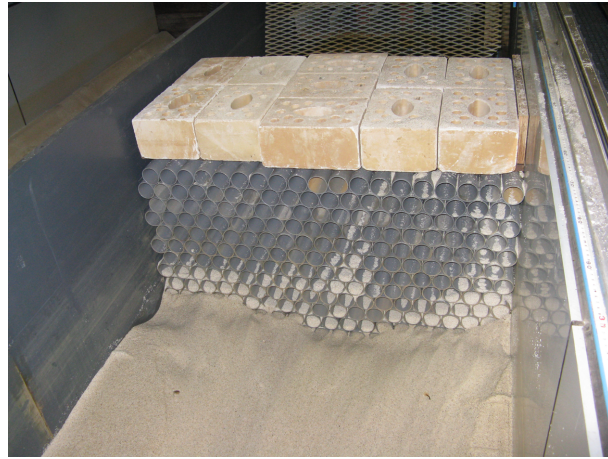
Photo 2.3 (above): Stacked tubes to reduce large scale turbulence from the water inlet tank and sediment recirculation.
