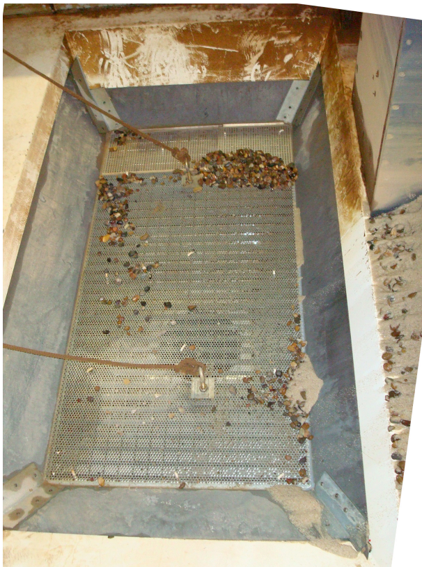
Photo 2.4: Gravel sieve in the sediment recirculation funnel.
