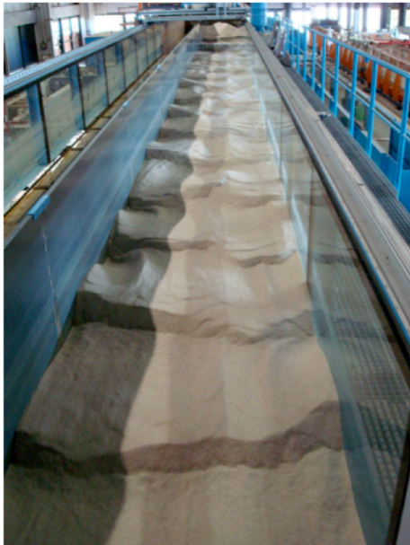
Photo 1.1: Dunes in an alluvial flume experiment. The flow direction was from top to bottom.
