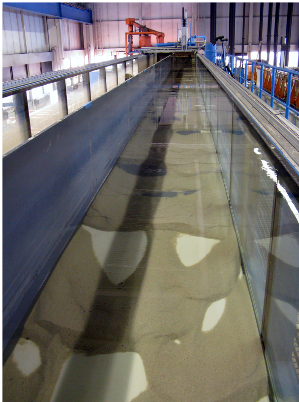
Photo 2.5: Bedforms formed on a smooth immobile layer.
